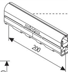
Barrier beam coupling clamp
