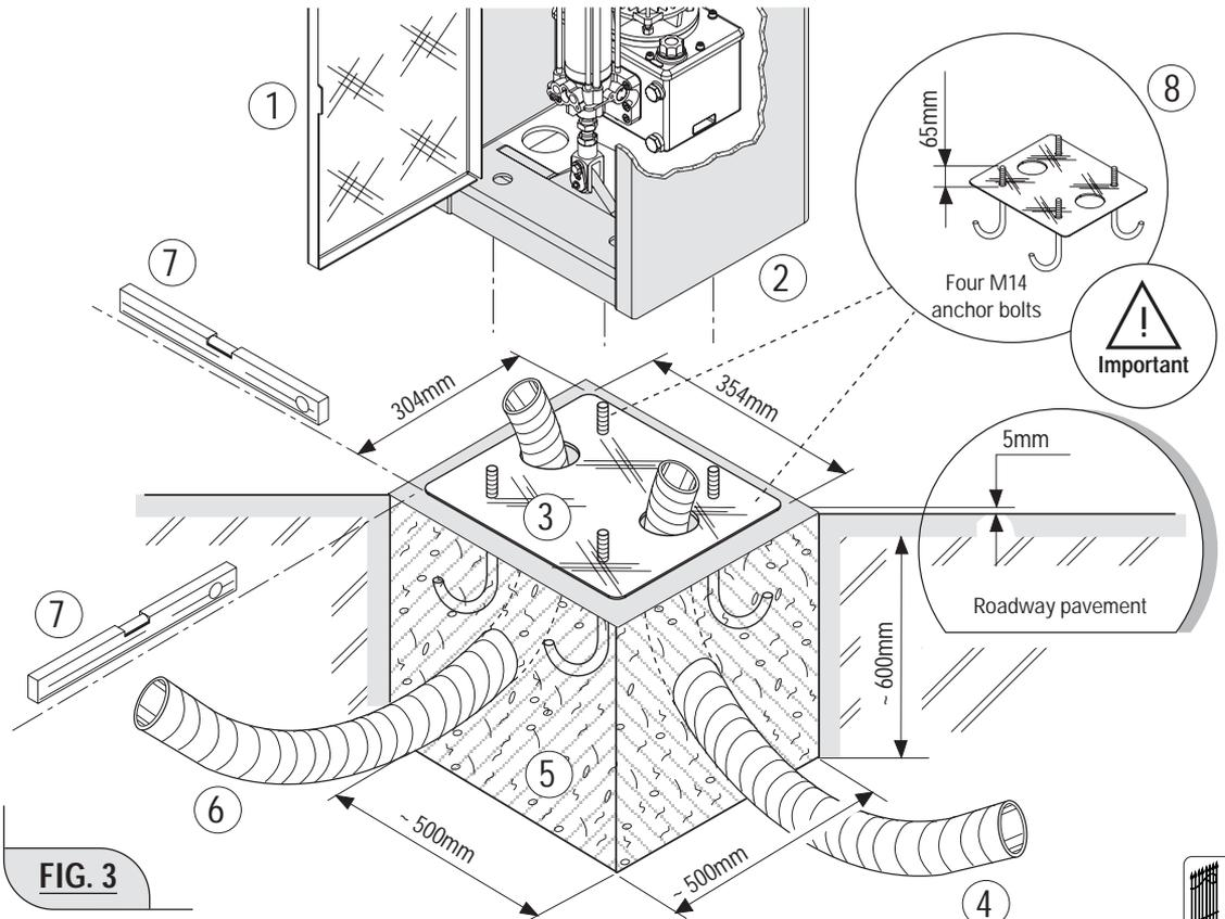
**Important:** screw down the entire length of the threading of the anchor bolts to the anchor plate before cementing it in its site.
