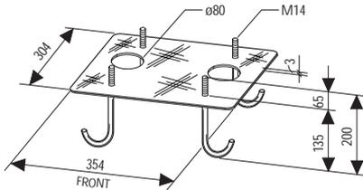
Anchor plate 354x200 with M14x200 galvanised anchor bolts.
