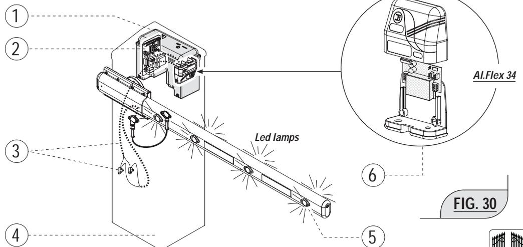
In the event of an installation of the Bayt 980 with **LED lamps** it is possible to connect the **Al.Flex 34** command device and to obtain the alternating flashing without pauses or else the alternating flashing of the "flash" type (Fig.30).
