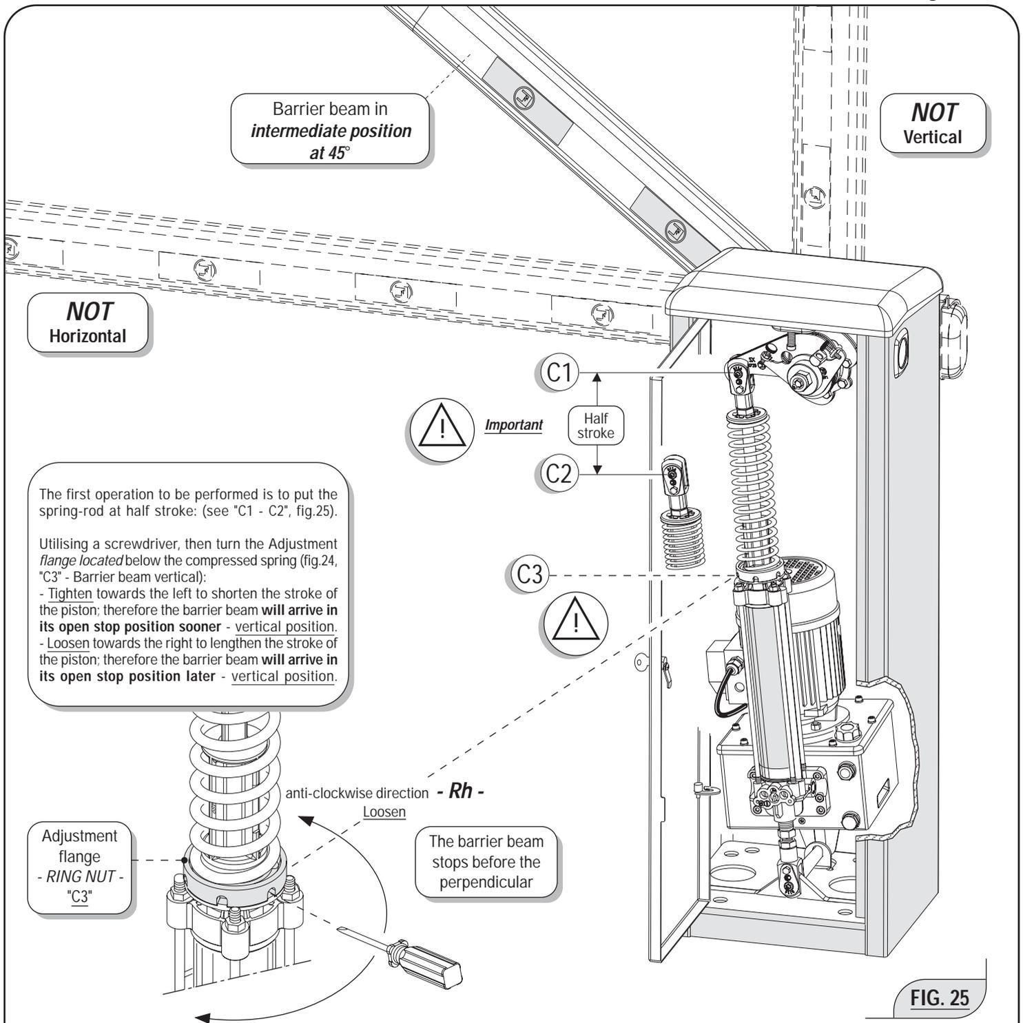
The first operation to be performed is to put the spring-rod at half stroke: (see "C1 - C2", fig.25).
