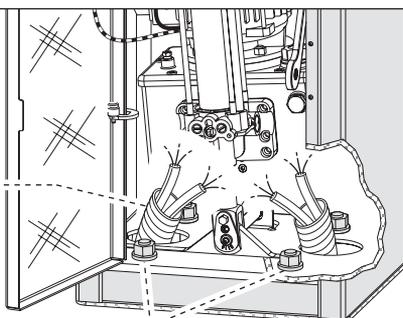
Tighten the four M14 hexagonal nuts with the washers supplied
