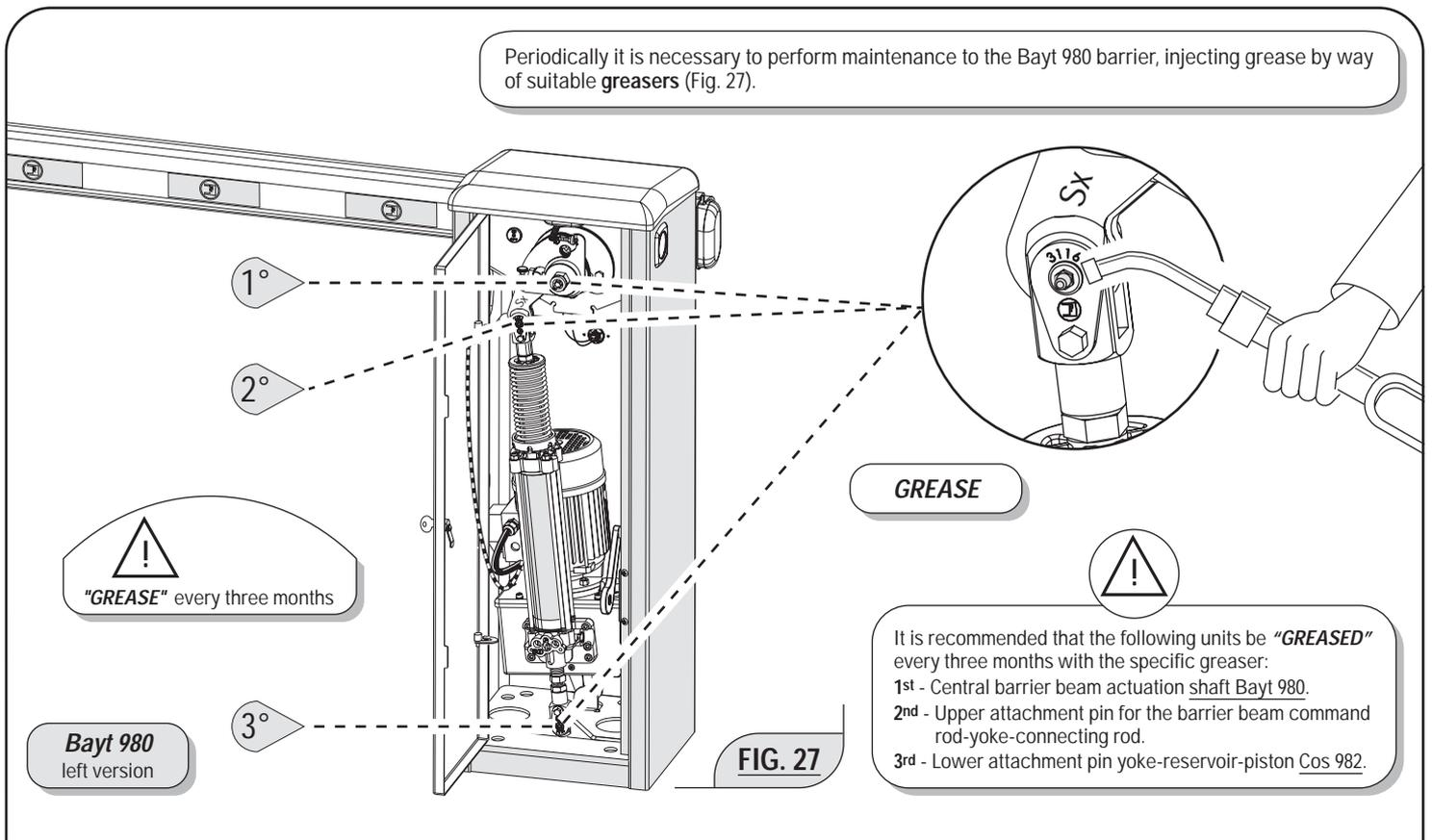
Periodically it is necessary to perform maintenance to the Bayt 980 barrier, injecting grease by way of suitable greasers (Fig. 27).
