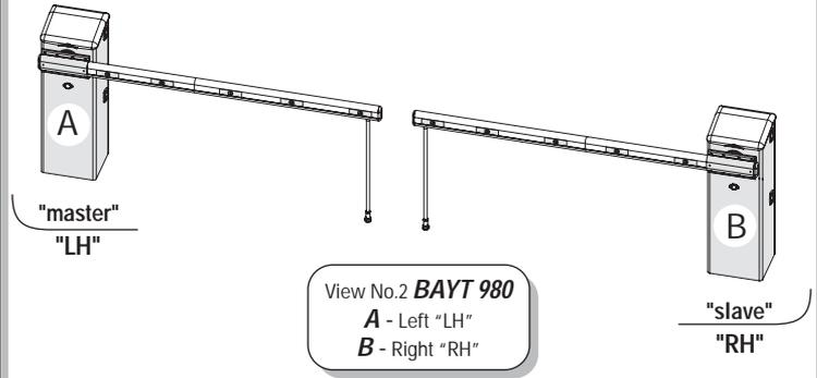
Before completing all of the electrical connections necessary, distinguish the Elpro 980 of the A "Master" Barrier, which commands the Elpro 980 in the B - "Slave" Barrier.
