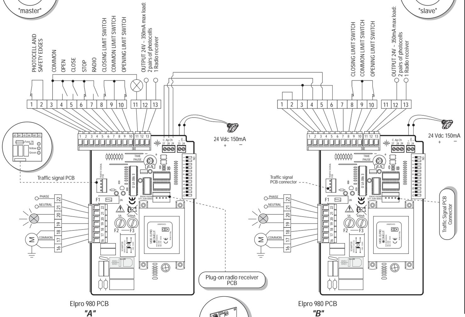
**IMPORTANT:** Any radio receiver or plug-on PCB for the traffic signal must be connected to the Master PCB A
