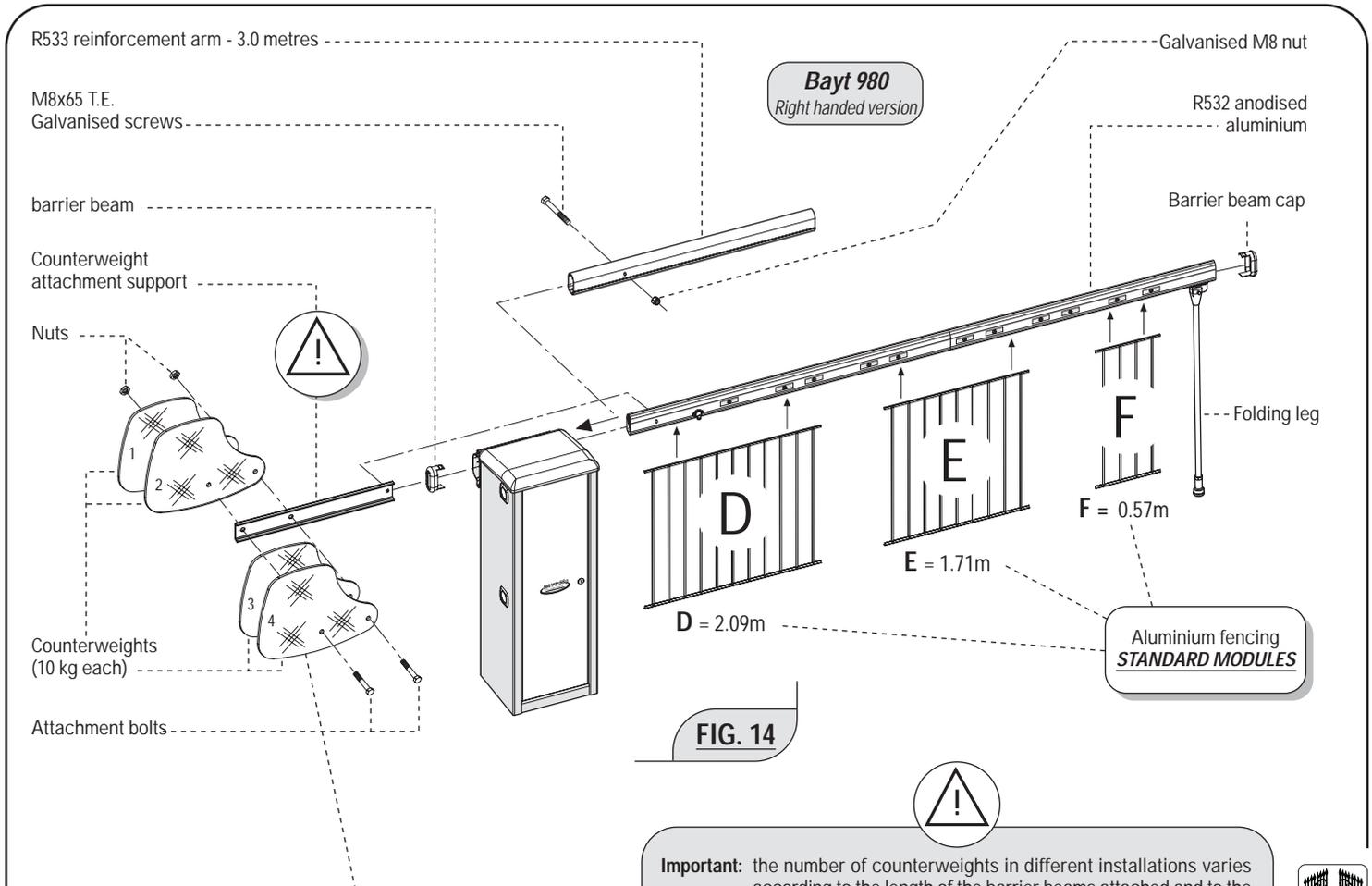
In the Bayt 980 installation with barrier beams that are 6.40 metres in length or longer with fencing, it is necessary to also attach **counterweights** with nuts, bolts and attachment support. (Fig. 14).
