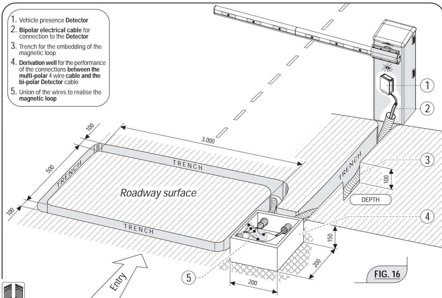
For the installations that require the utilisation of a **magnetic loop** it is recommended that the instructions found in Fig. 16 be followed, making reference to the connections indicated in Fig. 20 on Page 10 and on the instruction sheet attached to the magnetic loop. (Ref. Drawing 2126).
