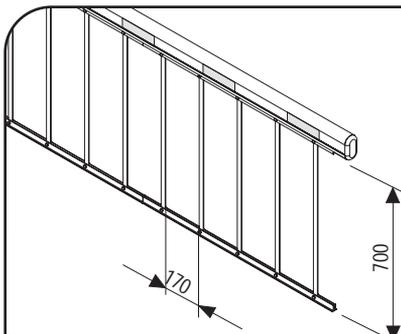
Aluminium fencing to be attached to the bottom of the barrier beam
