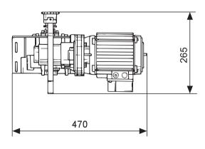
MEC 200 LB a chain drive motor reducer, has been designed to run gates made of sections, which are hinged together. The first section pulls all the others open and folds them at one end of the gate, so that they take up very little room.
